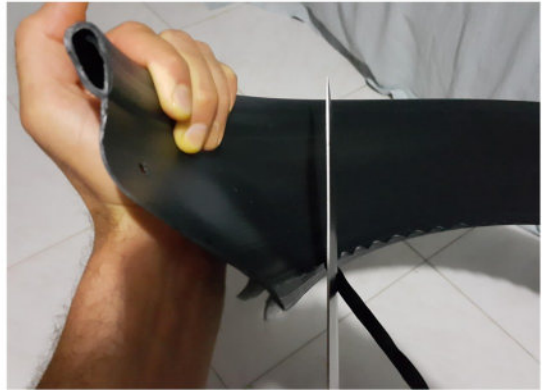
Remove plastic ridge inside the form
