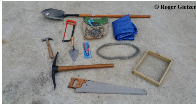
Reusable tools and supplies for constructing a vetiver latrine
